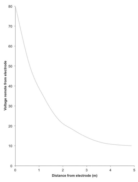
Figure 1 - Typical Voltage - Grandiet Distribution Curve
